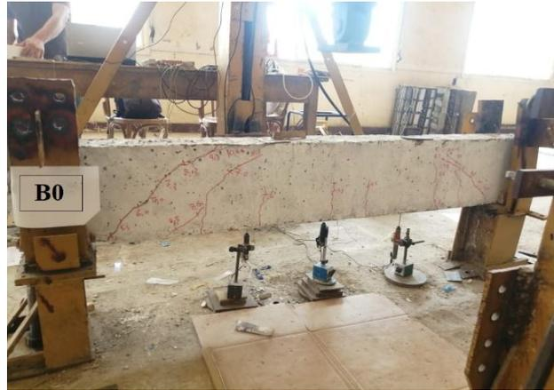
Fig. 14 Experimental and numerical comparison of specimen cracks
