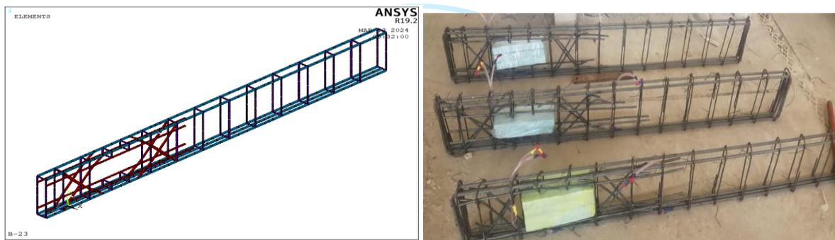
Fig.12 Beam reinforcement with diagonal bar surrounding openings
