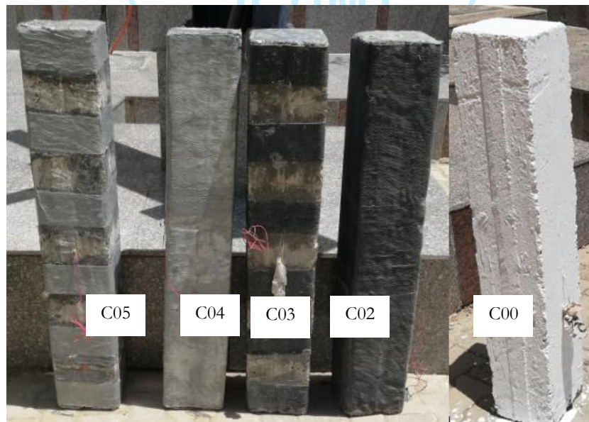
Fig. 2 Specimens after the formation of FRP jacket
