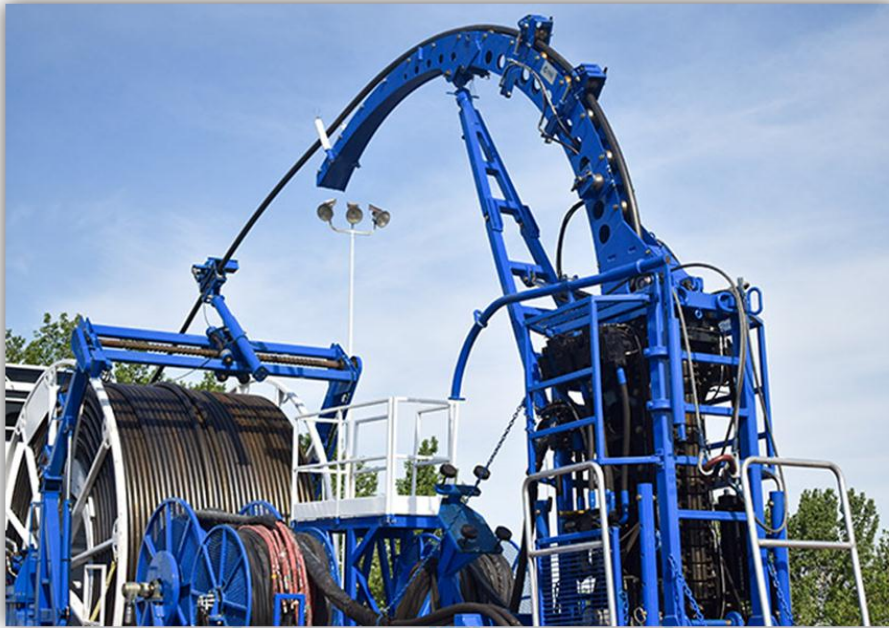
Fig. 2 Surfactant Injection through Coil Tubing [28]
