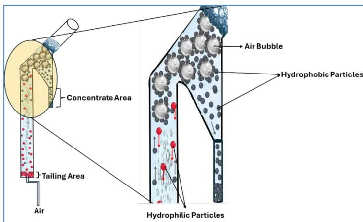
Fig. 2 Concept of Hallimond Micro-flotation tube
