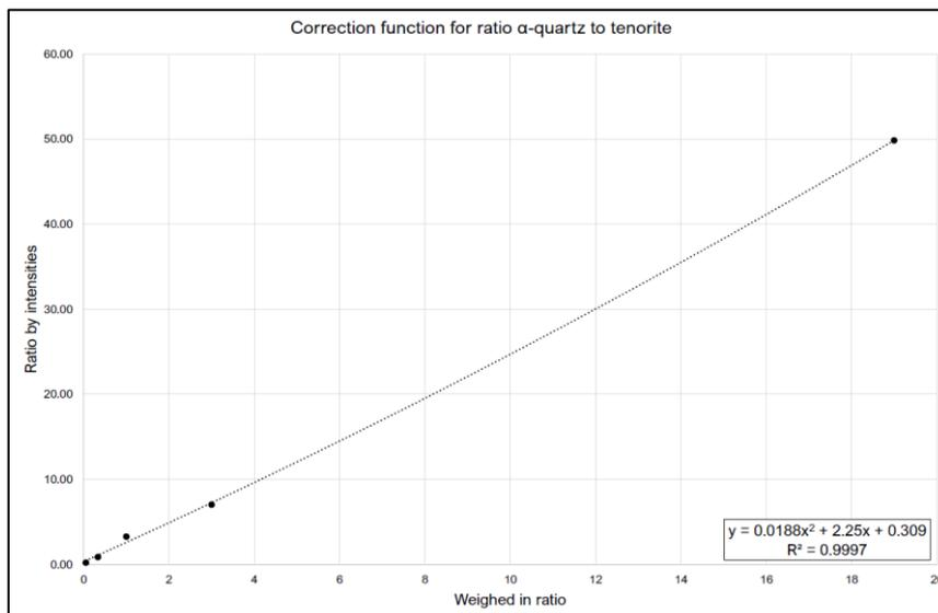
Fig. 1 Applied correction function with figure of merit based on mixtures with known fractions of quartz and tenorite.
