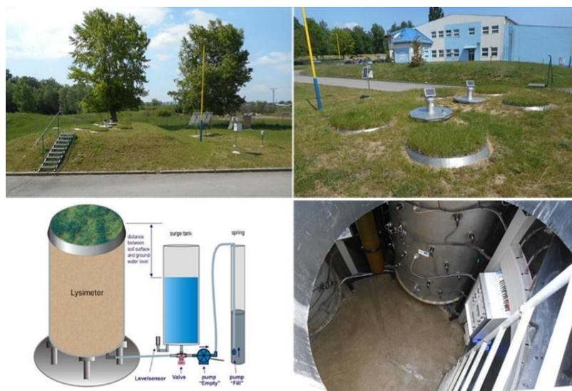
Fig. 2 Weighing lysimetric station for ET measurement
