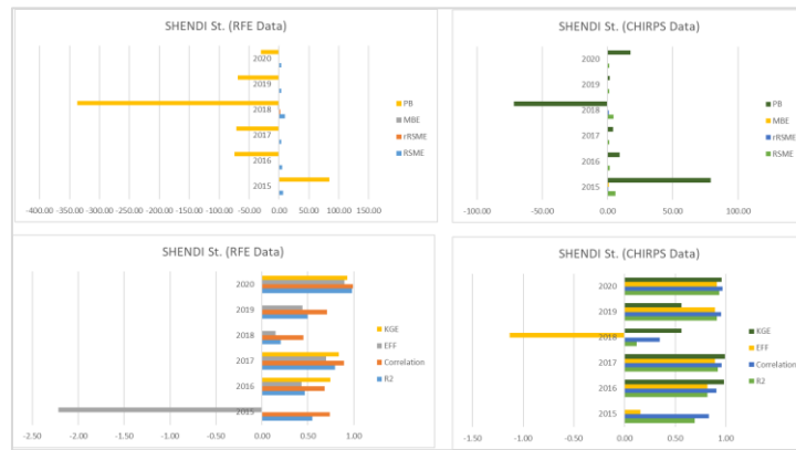
Fig. 10 performance measures metrics (R2, RMSE, rRMSE, MBE, PB, EFF, KGE) for observed meteorological stations against detected and estimated RFE2.0 and CHIRPS from January 2015 to December 2020.
