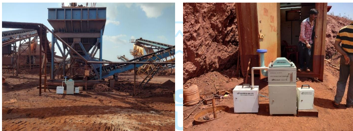
Fig. 8 Dust sampling using a respirable dust sampler (Ecotech AAS 190) ( \text{PM}_{10} ) and Particulate dust sampler (Ecotech AAS127) ( \text{PM}_{2.5} )
