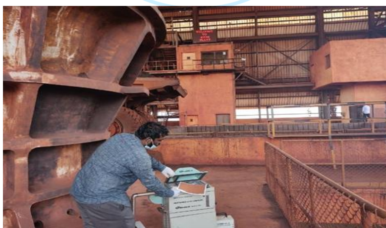
Fig. 8(a) High volume RDS sampler in crusher area
