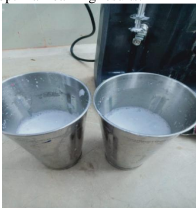
Fig. 15 Mixing Surfactants using Mud Mixer
