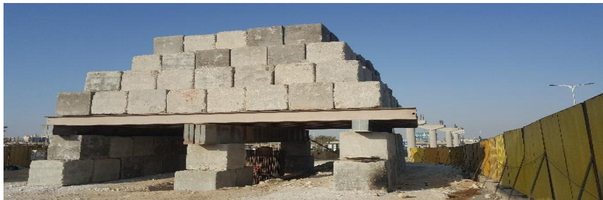
Fig. 4 Field photo of axial static load test, (The Arab Contractors, Foundation department, 2020)
